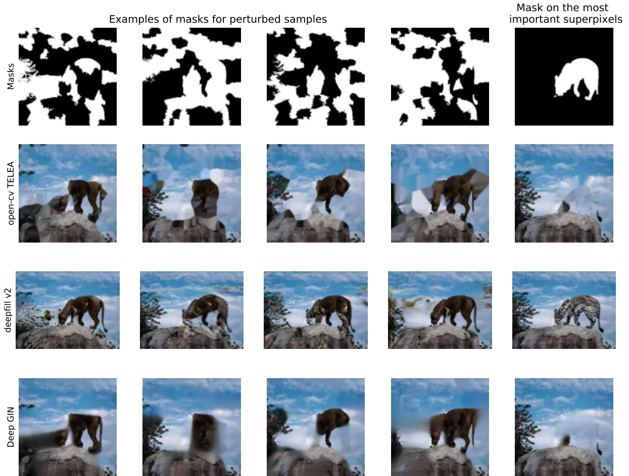
Figure 12: Comparison of three generative inpainting models on the image of a lion using different masks. The first row presents the masks, where the white parts determine the region of the image to be inpainted. The first 4 exemplify the type of masks that LIME-G uses to create perturbed samples. In the last column, the mask determines to inpaint the superpixels that contain the lion. Rows 2 to 4 show the results of the different inpainting techniques. DeepGIN provides the best results given that it succeeds on erasing the parts of the lion that are masked and replacing them with credible backgrounds.
