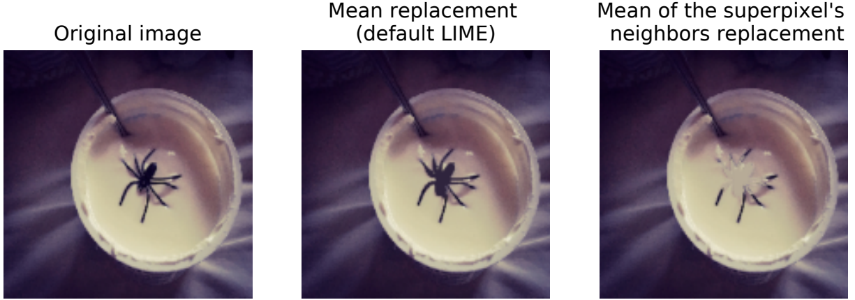
Figure 6: Using mean replacement (default LIME) and mean of the superpixel’s neighbors in an image where only the most important superpixel (the one containing the tarantula) is turned off . The original image is displayed on the left. The center image shows the effect of using mean replacement (default for LIME) for a single superpixel, resulting in little to no change compared to the original. The image on the right shows how using mean of the superpixel’s neighbors replacement manages to make the tarantula mostly “disappear.”
